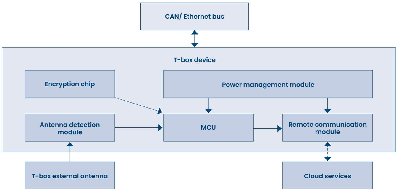
Figure 14 Reference architecture of the T-box system
