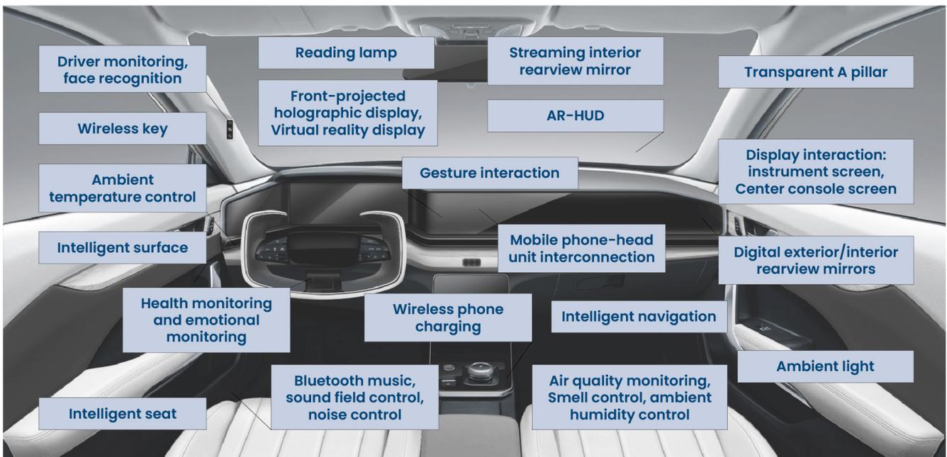
Figure 2 Technical diagram of an intelligent cockpit product
