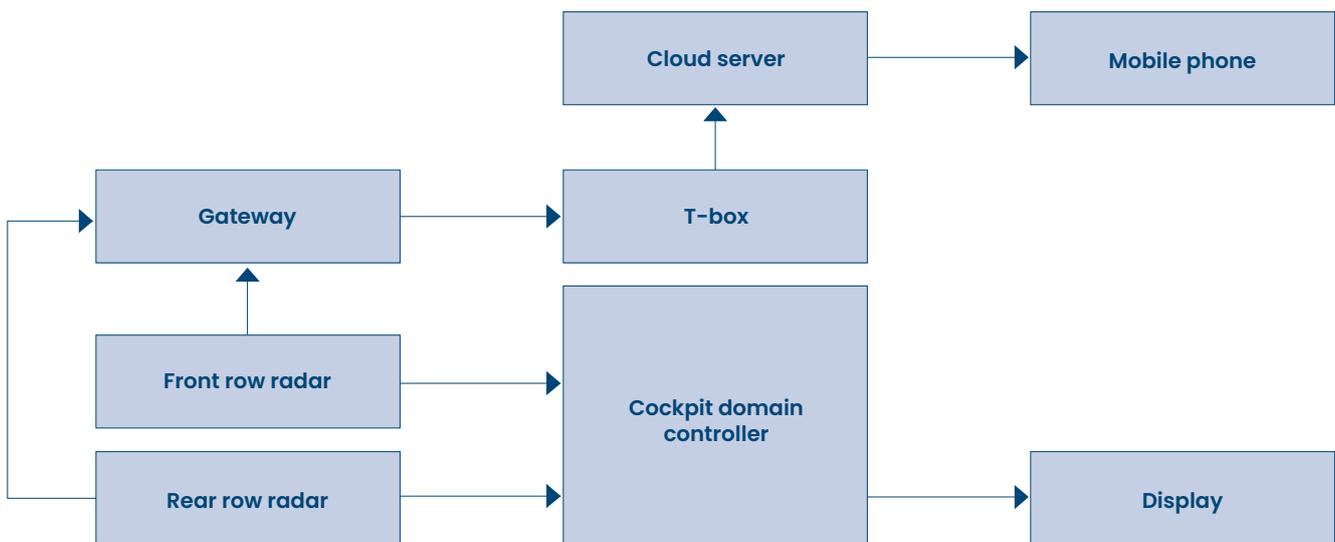
Figure 6 Reference architecture for an in-cockpit radar system
