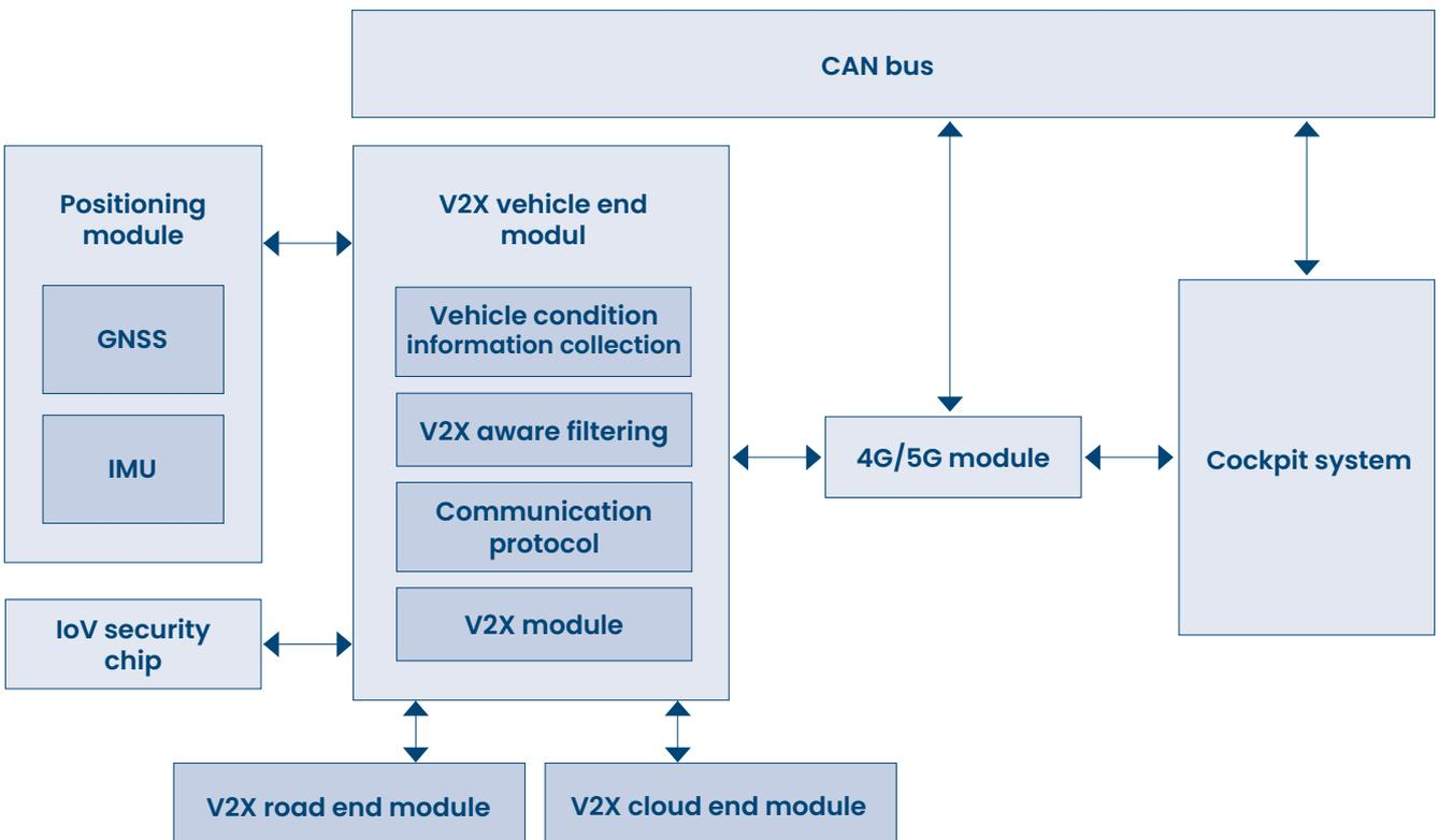
Figure 13 Reference architecture for the V2X vehicle end system
