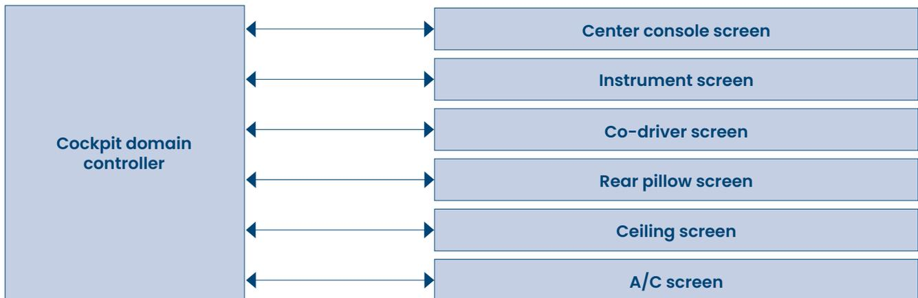
Figure 10 Reference architecture for the on-board display system
