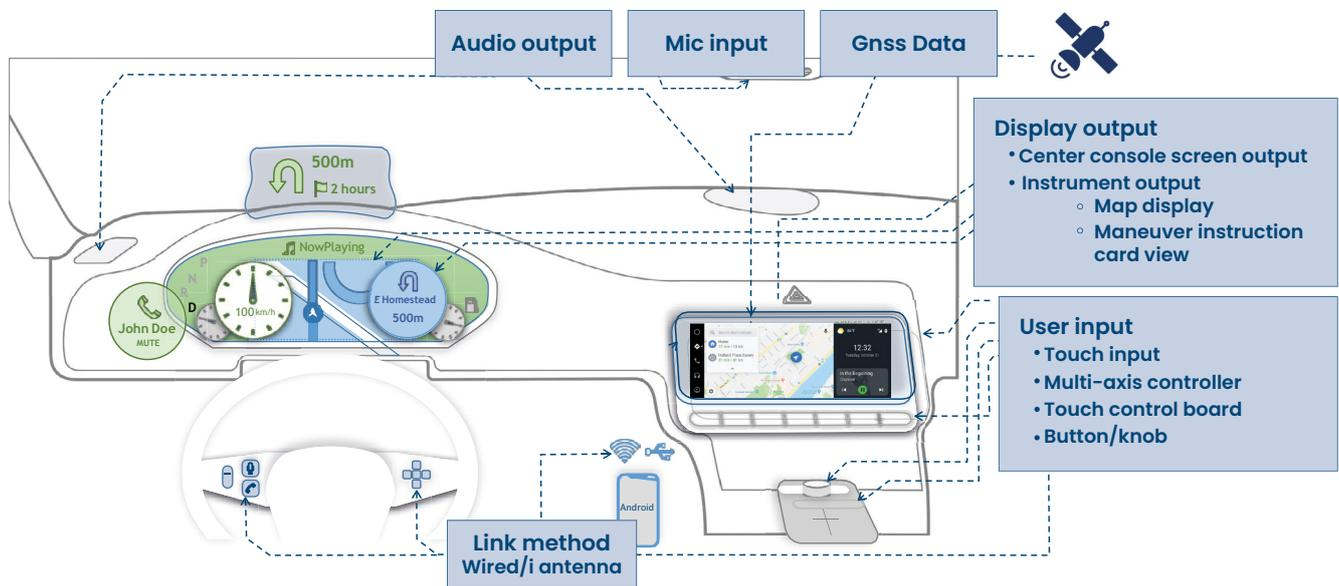
Figure 21 Principles of mobile phone screen projection technology
