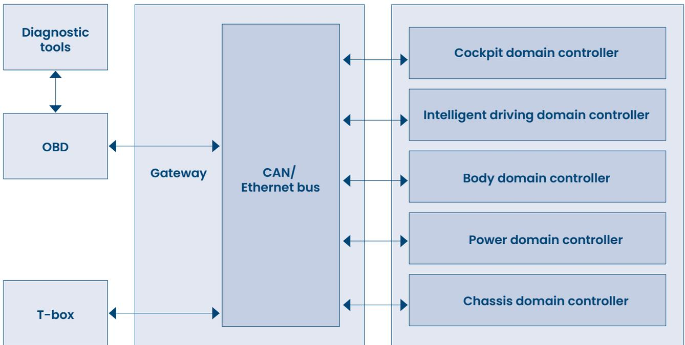
Figure 12 Reference architecture for the centralised gateway system
