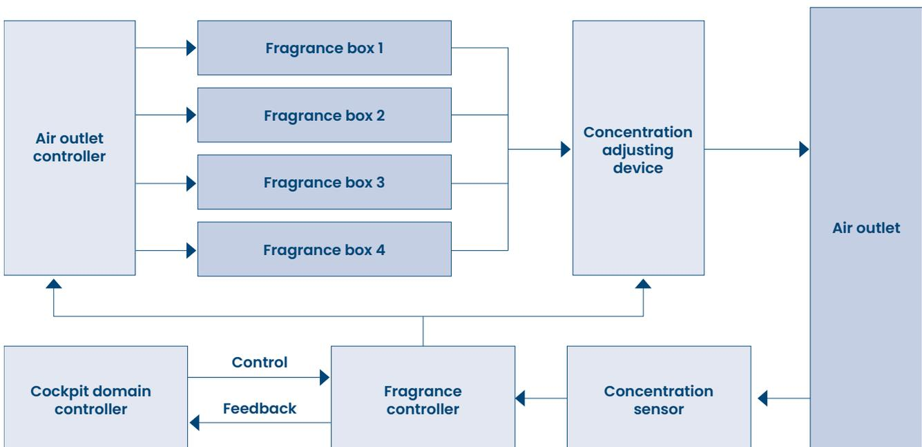
Figure 16 Reference architecture for the on-board fragrance system
