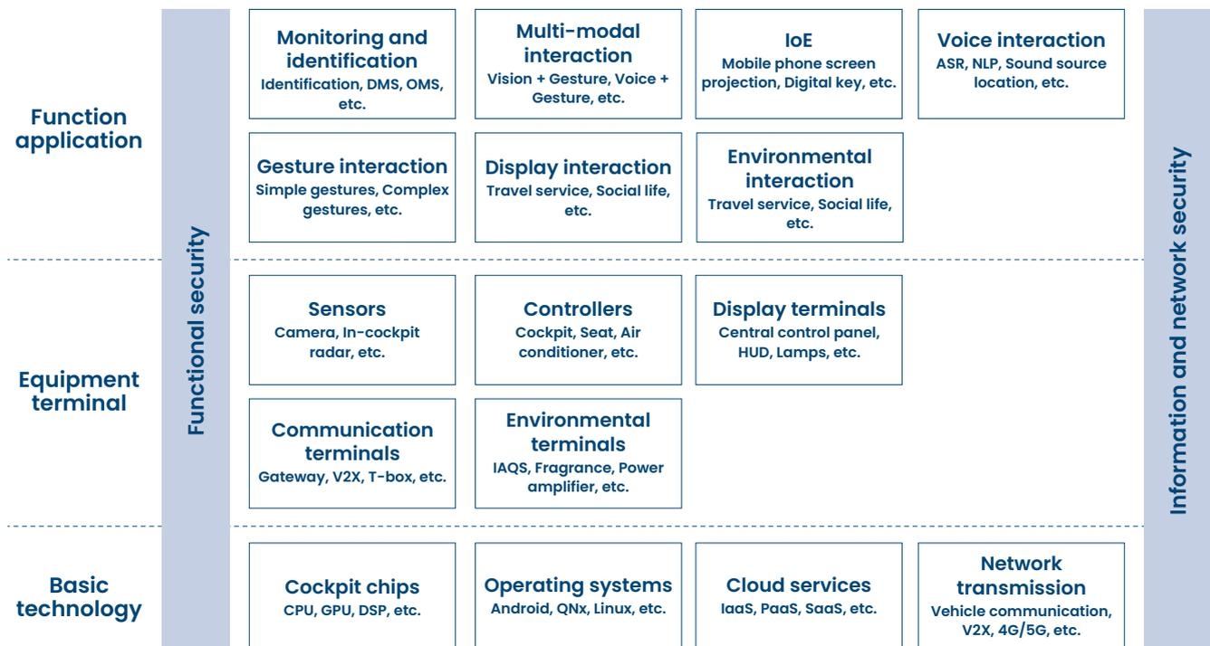
Figure 3 Reference architecture for the intelligent cockpit
