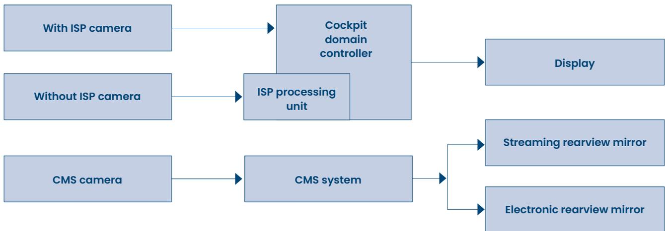
Figure 5 Reference architecture for a cockpit camera system
