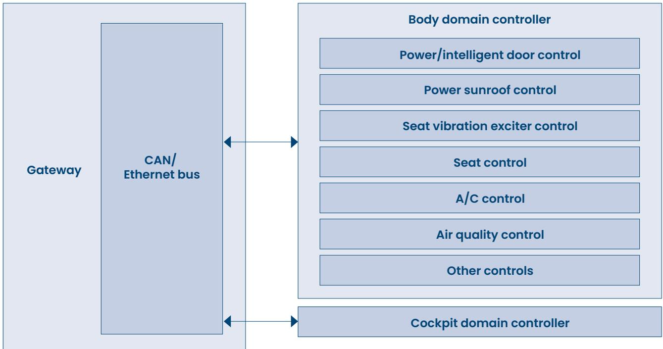
Figure 9 Reference architecture for the centralised body control system
