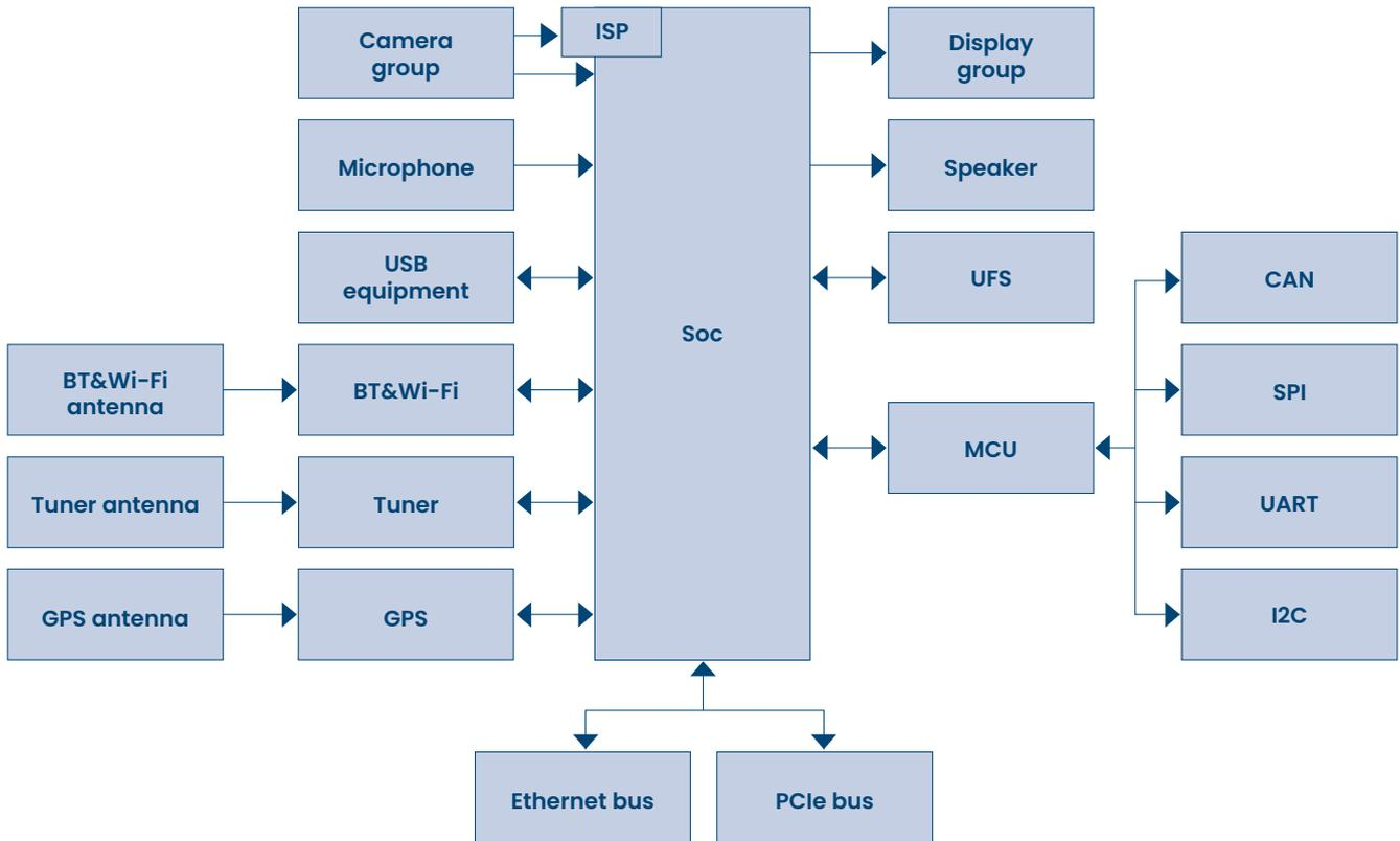
Figure 7 Reference architecture for the cockpit domain controller system
