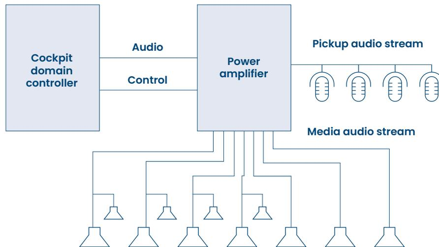
Figure 17 Reference architecture for the auto audio system (both internal and external power amplifiers are applicable)
