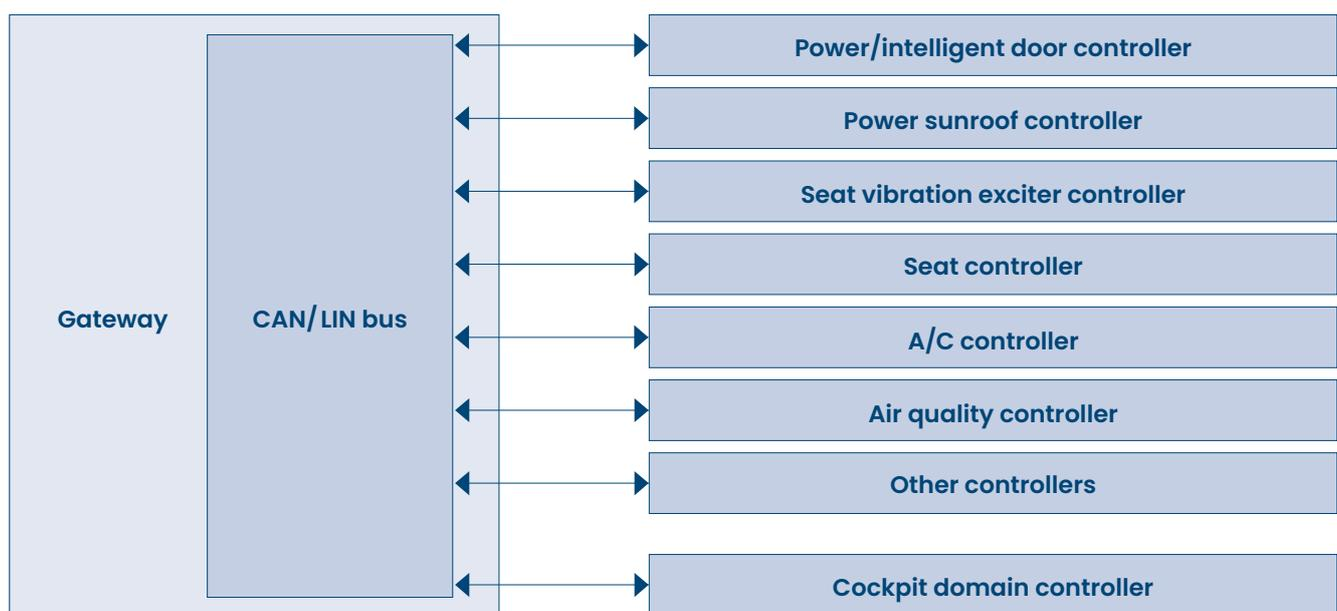
Figure 8 Reference architecture for distributed body control system
