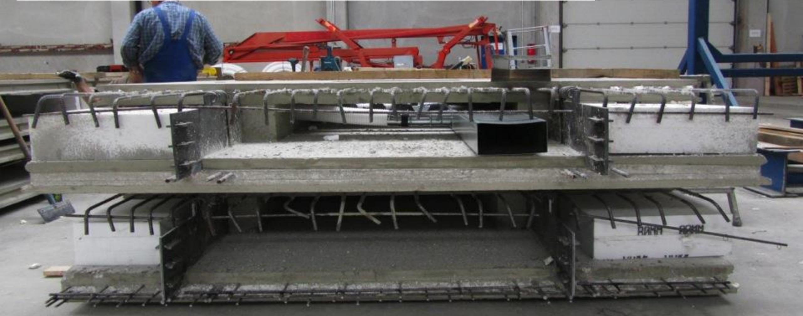
**Precast concrete elements:** all building service elements are installed within the precast plant and connected on site
