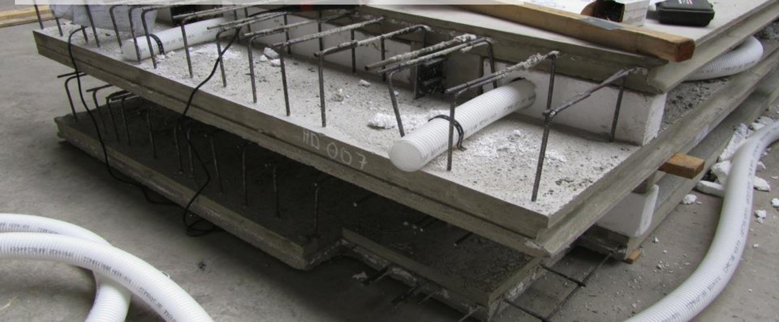
Service lines, pipes, tubes are integrated in the precast factory
