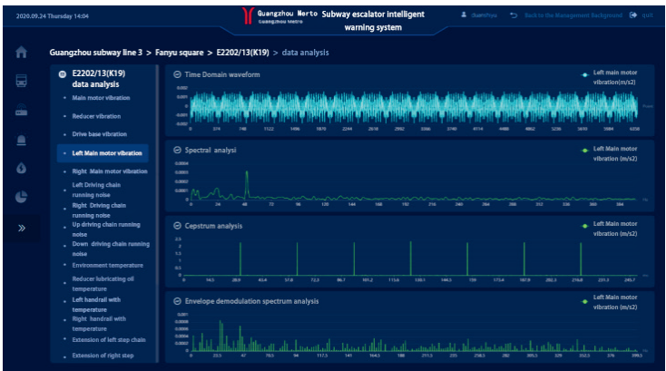
Figure 4-18-5 –Escalator condition monitoring and fault early warning system interface
