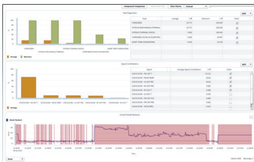
Figure 4-11-6 –Compressor predictive maintenance system failure analysis interface
